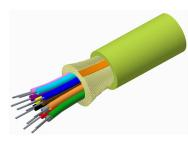
Fiber indoor cable, LazrSPEED® Low Smoke Zero Halogen Riser Distribution Cable, 4 fiber single-unit, Gel-free, Multimode OM5, Feet jacket marking, Lime green jacket color, B2ca flame rating
