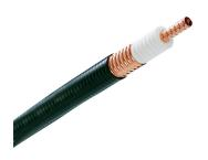
AVA7RK-50, HELIAX® Andrew Virtual Air™ Coaxial Cable, corrugated copper, 1-5/8 in, black non-halogenated, fire retardant polyolefin jacket Cca-s2, d2, a1 (CPR testing is conducted annually please reference the website for latest classification)
