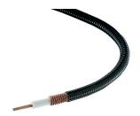
FSJ4-50B, HELIAX® Superflexible Foam Premum Coaxial Cable, corrugated copper, 1/2 in, black non-halogenated, fire retardant polyolefin jacket B2ca-sla,d1,a1
