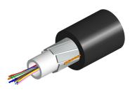
Fiber Indoor/Outdoor Drop Cable, TeraSPEED®, Low Smoke Zero Halogen, 18 fiber, Single Jacket All-Dielectric Arid-Core, Gel-filled, Singlemode + Multimode OM3, Feet jacket marking, Black jacket color, Dca flame rating
