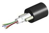
Fiber drop cable, TeraSPEED® Single Jacket All-Dielectric Arid Core, 12fiber, Singlemode G.652.D and G.657.A1, Gel-filled, Feet jacket marking, Black jacket color
