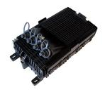
Mini-OTE 300-Series, Optical Terminal Enclosure, 4-port full-size connector, with integrated 1x4 splitter, black, with grounding, external mounting. Splitter outputs connected to terminal housing ports, maximum 26 splices.
