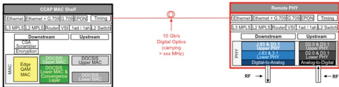
Figure 26: Remote PHY Architecture (RPA)
