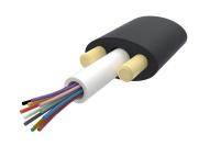
Fiber drop cable, Self-Supporting All-Dielectric, 12 fiber Arid Core construction, central loose tube, Gel-filled, Singlemode G.657.A2/B2, Meter jacket marking, Black jacket color
