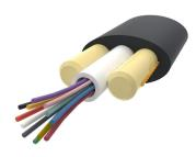
Fiber drop cable, Self-Supporting All-Dielectric, 4 fiber Arid Core construction, central loose tube, Gel-filled, Singlemode G.657.A2/B2, Meter jacket marking, Black jacket color
