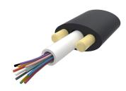
Fiber outdoor drop cable, LightScope® ZWP Self-Supporting All-Dielectric, Singlemode G.652.D and G.657.Al, 24 fiber, Arid Core construction, Gel-filled, central loose tube, no ripcords, Feet jacket marking, Black jacket color
