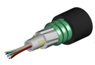
Fiber drop cable, LightScope® ZWP Single Jacket Single Armor Outdoor Drop Cable, 2 fiber Arid Core construction, central loose tube, Gel-filled, Singlemode G.652.D and G.657.Al, Meter jacket marking, Black jacket color
