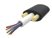
Fiber outdoor drop cable, LightScope® ZWP Self-Supporting All-Dielectric, Singlemode G.652.D and G.657.Al, 4 fiber Arid Core construction, Gel-filled, central loose tube, Feet jacket marking, Black jacket color
