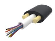
Fiber outdoor drop cable, LightScope® ZWP Self-Supporting All-Dielectric, Singlemode G.652.D and G.657.Al, 6 fiber Arid Core construction, Gel-filled, central loose tube, Feet jacket marking, Black jacket color
