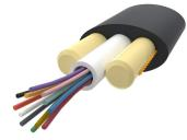
Fiber outdoor drop cable, LightScope® ZWP Self-Supporting All-Dielectric, Singlemode G.652.D and G.657.A1, 6 fiber Arid Core construction, Gel-filled, central loose tube, Meter jacket marking, Black jacket color
