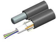
Fiber outdoor drop cable, LightScope® ZWP Self-Supporting Non-Armored Figure-8, Singlemode G.652.D and G.657.A1, 2 fiber Arid Core construction with 0.109 in messenger, Gel-filled, central loose tube, Feet jacket marking, Black jacket color
