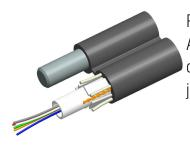
Fiber outdoor drop cable, LightScope® ZWP Self-Supporting Non-Armored Figure-8, Singlemode G.652.D and G.657.A1, 6 fiber Arid Core construction with 0.109 in messenger, Gel-filled, central loose tube, Feet jacket marking, Black jacket color
