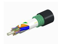
Fiber indoor/outdoor cable, LightSCOPE® Indoor/Outdoor, Single Jacket /Single Armor, Low Smoke Zero Halogen (LSZH), Singlemode G.652.D and G.657.A1, 48 fiber, Gel Filled, Stranded Loose Tube, Meters jacket marking, Black jacket color, Cca flame rating
