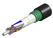
Fiber OSP cable, LightScope® ZWP Mini Single Jacket/Single Armor, 6 fiber, Gel-Filled, Stranded Loose Tube, Singlemode G.652.D and G.657.Al, Meters jacket marking, Black jacket color
