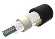
Fiber OSP Cable, Non-Armored, All-Dielectric, Arid-Core, Dry Central Tube Ribbon, 12 fibers, Singlemode G.652.D and G.657.A1, Gel-free, Feet jacket marking, Black jacket color
