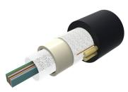
Fiber OSP Cable, Non-Armored, All-Dielectric, Arid-Core, 48 fibers, Dry Central Tube Ribbon, Singlemode G.652.D and G.657.Al, Gel-free, Feet jacket marking, Black jacket color
