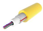
Indoor/Outdoor Fiber Optic Cable, loose tube, 12-fiber, OS2, singlemode, LSZH, dielectric, yellow. Provides Rodent Resistance.
