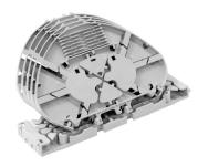
FIST® Splice Sub-assembly kit with 5 trays, each for holding up to 12 primary or 4 secondary coated fibers, with ANT type splice holder
