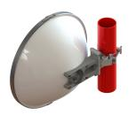
0.6m | 2ft ValuLine High Performance Antenna, dual polarized, 31.000 – 33.400 GHz, PBR320 Flange, White Antenna, Grey Radome
