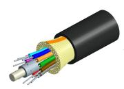
Fiber Indoor/Outdoor cable, OptiSPEED® Low Smoke Zero Halogen Riser Distribution, Gel-Free, 4 fiber single-unit, Multimode OM1, Feet jacket marking, Black jacket color, Dca flame rating
