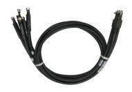
HELIAX® M-LOC Multiport cluster 5 ports SureFlex® cable assembly with interface type M-LOC latching male to 4.3-10 male, size 3/8", length 2 meters, covered by conduit shield
