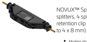
NOVUX™ Specialty Range Closure 10, splice only, no adapters, no splitters, 4 splices, SMOUV® 45mm splice protectors, black, 2x CR cable retention clip (Round cable : Range 4 to 6.2 mm & Flat cable : Range 3 x 5 to 4 x 8 mm)
